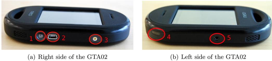
**Figure 1.3:** (a) On the right side of the GTA02, the power button, an USB connector and an external GPS antenna connector. (b) On the left side of the GTA02, the ‘aux’ button and a 2.5mm phone jack connector. (Pictures from <http://wiki.openmoko.org>)
